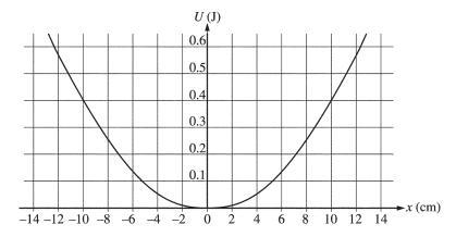
A 3.0 kg object subject to a restoring force F is undergoing simple harmonic motion with a small amplitude. The potential energy U of the object as a function of distance x from its equilibrium position is shown above. This particular object has a total energy E of 0.4 J.
