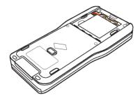
5. Replace the back panel and fasten the screws with a screwdriver.
