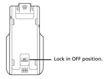
To attach the handheld, face the screen upward and slide the handheld onto the top of the TI-Nspire™ Navigator™ wireless cradle. Be sure that both sides of the handheld are inserted into both of the side guides.
