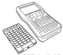
TI-84 Plus keypad (on left) and TI-Nspire<sup>TM</sup> keypad (on the handheld)
