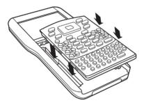
Push the keypad firmly into place. You will hear a click and the switch on the back of the keypad is in the locked position.
