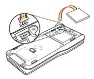
4. Thread the wire into the case to secure it. Insert the rechargeable battery into its compartment.
