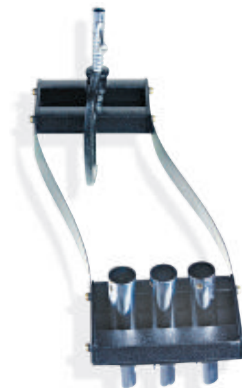
■ Figure 7-13 An inertial balance allows you to calculate the inertial mass of an object from the period ( T ) of the back-and-forth motion of the object. Calibration masses, such as the cylindrical ones shown here, are used to create a graph of T^2 versus the mass. The period of the unknown mass is then measured, and the inertial mass is determined from the calibration graph.
