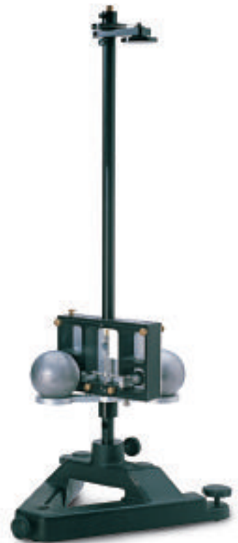
■ Figure 7-6 Modern Cavendish balances are used to measure the gravitational forces between two objects.
